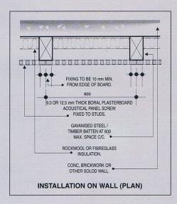
**BORAL PLASTERBOARD ACOUSTICAL** panels are lay-in type ceiling panels to be used on exposed suspended ceiling grids. The panels are also suitable for internal wall linings. The panels have a surface finished in proprietary white emulsion paint specially formulated for maximum protection and good light reflectance properties.
